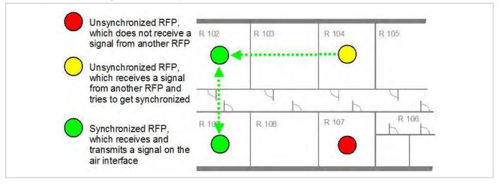
As long as an RFP is not in sync, no calls can be established using this RFP.
