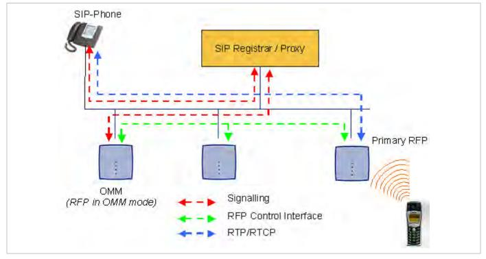
To establish a call between two DECT phones, the same IP streams must be established like in the scenario before, except the IP phone is not involved. The following figure illustrates this scenario.
