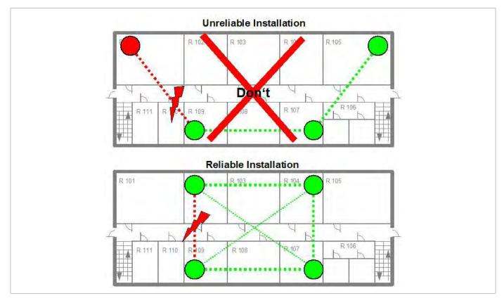
The sync-over-air solution is very reliable because all existing redundant paths are used for synchronization. Thus, hardware tolerances have only very little influence. No RFP has a key position.
