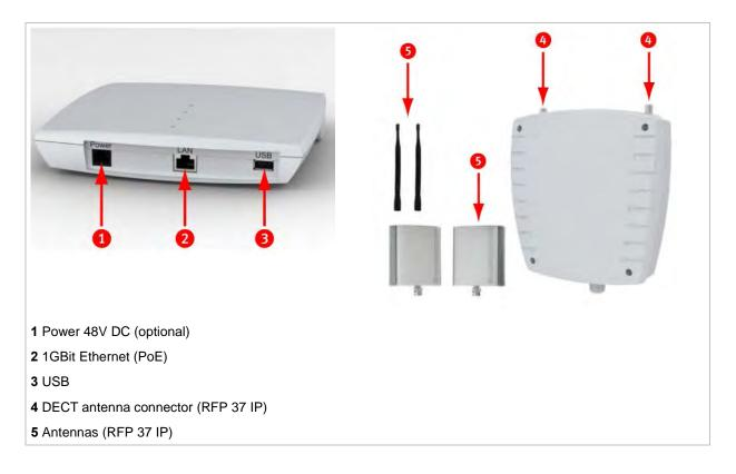
The hardware of all the new RFPs complies with the different regulatory domains. There are no specific hardware variants required to use specific frequency bands and field strengths. Transmit Power, frequency band and carrier frequencies are controlled by software.
