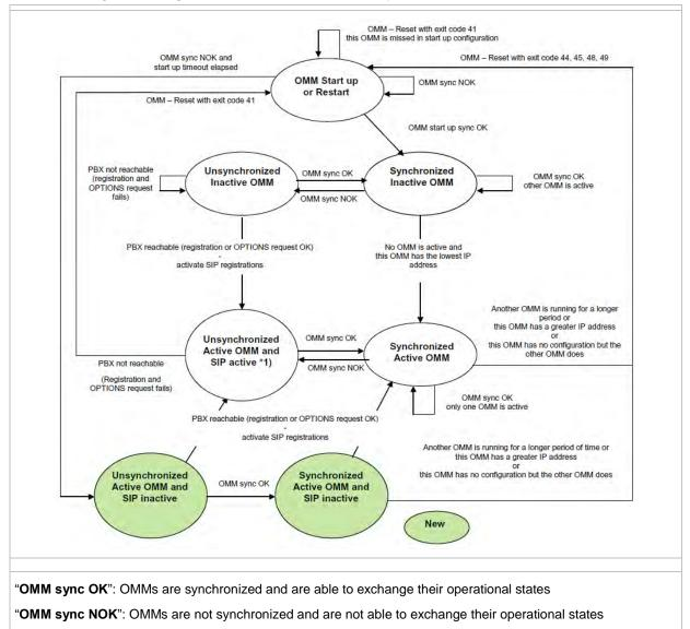
\*1) In this state the DECT air interface might not be in a definite state as both OMMs are active but cannot connect with each other! This is caused by IP network failures and cannot be handled by the SIP-DECT system in a proper automatic way. In such a scenario it is not predetermined which RFP connects with which of the 2 OMMs. The DECT network can split-up into two unsynchronized DECT sub-networks. This can cause voice quality and handover problems.
