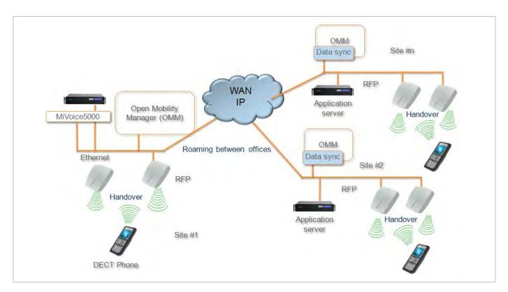
Instead of subscribing to the standard Primary Access Rights Key (PARK) of a single OMM when registering with the system, the DECT phones subscribe using the Secondary Access Rights Identifier (SARI) that applies to multiple OMMs in the system. All DECT phones that are subscribed to the system using the SARI can roam between sites (and OMMs). The PARK of the central OMM is defined to be the SARI.
