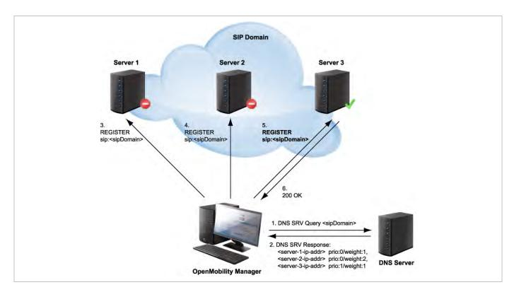
To prevent situations where the OMM tries to contact with each new transaction servers which are unreachable (out of service), the OMM offers a blacklist feature. If there is no answer from a SIP server, this specific server can be put into a blacklist and will not be contacted anymore for a configurable time of "Blacklist time out" minutes by all adjacent SIP transactions.
