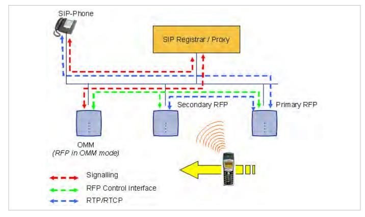
As the DECT phone user moves into the next RFP zone of coverage, the DECT phone detects that the RFP has a better signal strength. Again the media stream from the SIP phone cannot move to the secondary RFP, so the primary RFP uses the LAN to direct the voice to the new secondary RFP.
