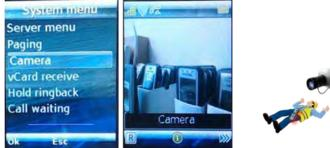
Video Streaming is only available when the DECT phone is connected to a RFP 35/36/37/43 and the permission is set for the site and the DECT phone.
