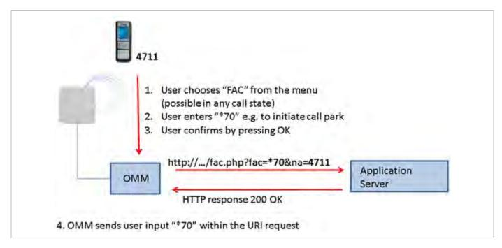
This feature can be configured using OMP on the XML applications page (see section 6.12.6).
