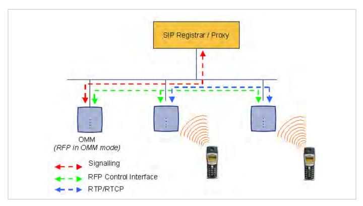
A call from one DECT phone to another that resides on the same RFP will loop back within the RFP if no media gateway is involved. So the call will not pass through to the Local Area Network (LAN). Although the voice packets will not impact LAN traffic, signal packets will.
