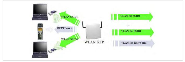
The access point can be assigned to a VLAN that conforms to 802.1q. All the data that is received from and that is to be forwarded to the WLAN clients is then carried by the configured VLAN. All other data, such as VoIP packets, configuration data or authentication data (Radius), is given the VLAN tag configured for the RFP. The switch port of the network component to which the access point is connected must be configured as a trunk port.
