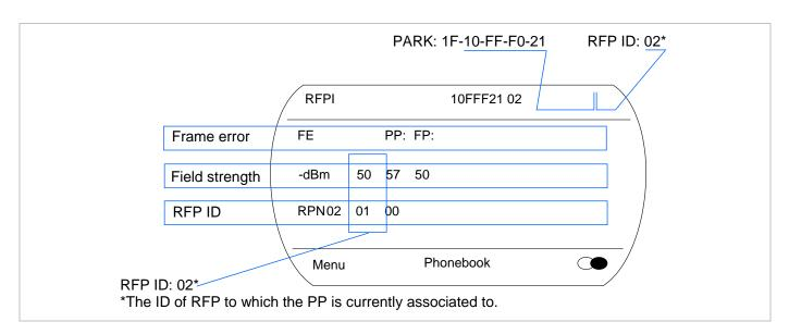
In this example the DECT phone is currently connected to the RFP with the number 02. The RFPs 01 and 00 are also visible. The number "10FFF221 02" on the upper right side refers to the PARK (Example 1F-10-F2-21) of the SIP-DECT system and to the RFP to which the phone is currently connected to.
