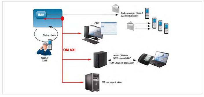
**IMPORTANT**: To address customer specific requirements, external applications (e.g. 3rd party software) can provide an addapted functionality of the user monitoring or even more just by using OM AXI. This can be completed by the use of the XML terminal interface.
