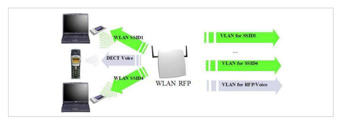
The access point can be assigned to a VLAN that conforms to 802.1q. All the data that is received from and that is to be forwarded to the WLAN clients is then carried by the configured VLAN. All other data, such as VoIP packets, configuration data or authentication data (Radius), is given the VLAN tag configured for the RFP. The switch port of the network component to which the access point is connected must be configured as a trunk port.
