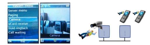
Video Streaming is only available when the DECT phone is connected to a RFP 35 and the permission is set for the site and the DECT phone.
