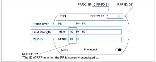
In this example the DECT phone is currently connected to the RFP with the number 02. The RFPs 01 and 00 are also visible. The number "10FFF221 02" on the upper right side refers to the PARK (Example 1F-10-F2-21) of the SIP-DECT system and to the RFP to which the phone is currently connected to.
