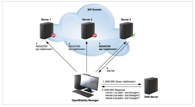
To prevent situations where the OMM tries to contact with each new transaction servers which are unreachable (out of service), the OMM offers a blacklist feature. If there is no answer from a SIP server, this specific server can be put into a blacklist and will not be contacted anymore for a configurable time of "Blacklist time out" minutes by all adjacent SIP transactions.
