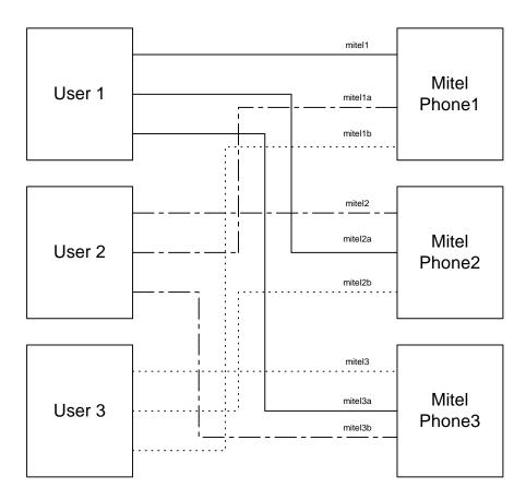
Figure 5: Shared Line Keys and User Configuration
