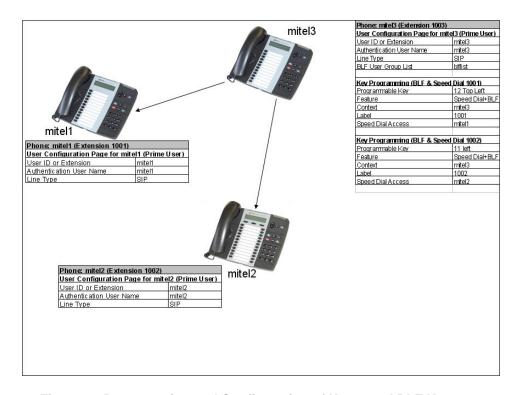
Figure 8: Programming and Configuration of Users and BLF Keys
