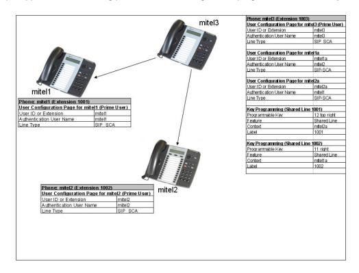
Figure 6: Programming and Configuration of Users and Shared Line Keys
