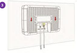
For wall or ceiling mounting connect the cables to the Enterprise Cell before mounting the Enterprise Cell on the stand
