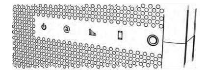
Power: Red – the Enterprise Cell is powered on Flashing red – a problem has been detected, please contact your service provider
