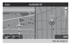
The change of direction is performed when the light-colored bar on the right drops down to 0 ft and the current vehicle position symbol has reached the white change-of-direction point
