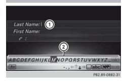
In the example, a new entry is added to the phone book (> page 100). The new entry has three input lines for entering the last name, first name and phone number. The input line for the surname is selected automatically.
