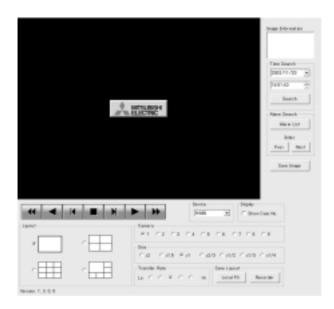
The date and time and the camera number for the image acquired are displayed in "Image Information". Clicking "Save Image" stores the picture that is freeze-frame displayed in the PC in bit map format.
