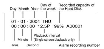
This unit displays the used space of the specified recording device (HDD) on the screen when "REMAIN HDD" of the <REAR TERMINAL SETTINGS> screen is set to "MAIN", "SUB". The "%" indicates the ratio detected as HDD against the total HDD capacity. The following settings are required to enable this function.
