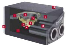
High-efficiency designed 20 cm woofer unit — 2. IMPP Cone — 3. Large-sized Strontium magnet — 4. Four-layer long voice coil — 5. Large diameter Conex damper — 6. Projected pole yoke — 7. Ported chamber — 8. Built-in 100 W amplifier with large Aluminum heat sink — 9. Sealed chamber — 10. Rigid carpeted wooden enclosure — 11. Large dual port
