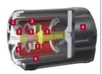
1. Aluminium frame - 2. Ring port - 3. Precision Triple Damper - 4. High density resin cabinet - 5. Foam IMPP Drive Cone - 6. Foam PP side wall - 7. Mid-ship mount magnetic circuit with large magnet
