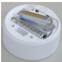
When installing the battery cover, insert the edge with the two tabs first and then press the cover into its recess until it clicks into place.
