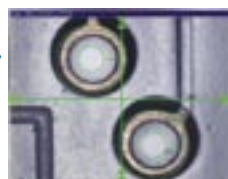
3. As the green cross-hairs approach the red cross-hairs the next measurement point comes into the screen.
