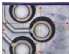
2. Move the stage to place the green cross-hairs on top of the red cross-hairs.
