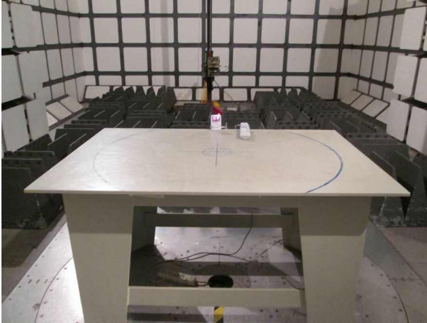
Radiated Emissions - Front View (Above 1 GHz)
