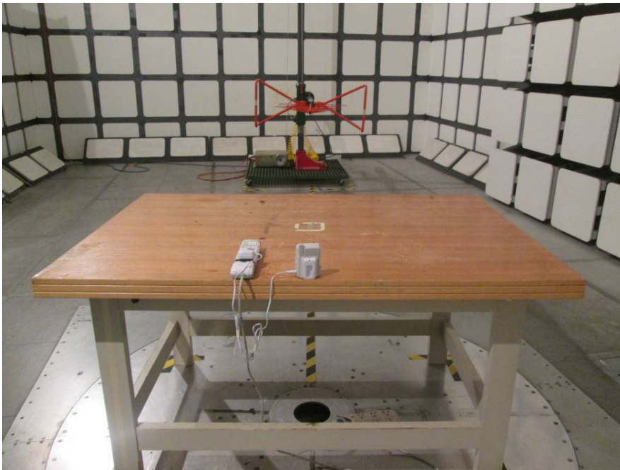
Radiated Emissions - Rear View (Below 1 GHz)
