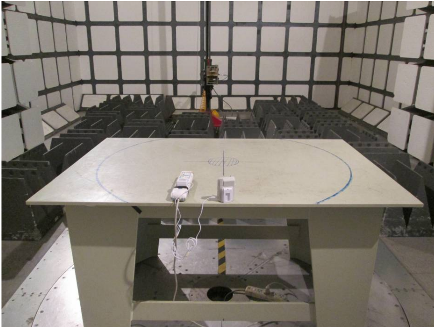
Radiated Emissions - Rear View (Above 1 GHz)
