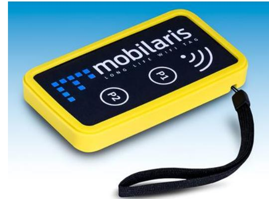
The long-life personnel tag is equipped with a powerful battery with a life cycle of up to three years (depending on transmission rates and other configurable parameters).
