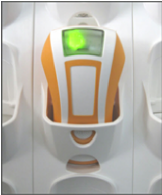
Charged Tag in Power Dock
