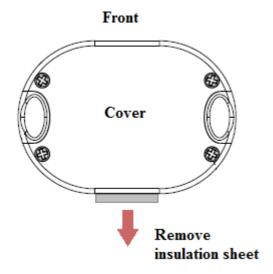
The device comes with a battery pre-inserted. Before using the device, the insulation sheet must be removed in order to use the device.
