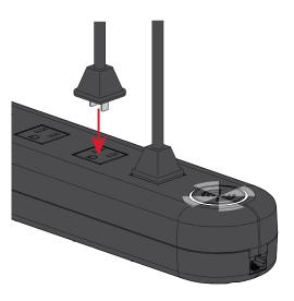
4 When all products have been successfully setup, plug cables back into product end at this time. Apply an "Alarm" label to product end of cable, if desired.
