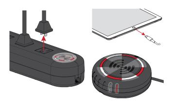
4 Placing a User Key over the RFID icon will silence the alarm. The LED will remain flashing red/white.
