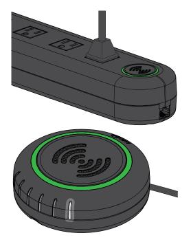
If unsuccessful → unit beeps 4 times and LED will be solid red. The Remote Access Module will show a corresponding red LED for that socket port. Unplug cable from the Power Strip and try again making sure cables are unplugged from the product.
