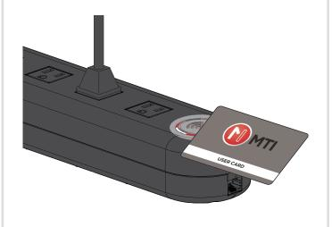
**5** To re-arm, fix the issue by plugging all cables back in. Place a User Key over the RFID icon and the LED will be solid white.
