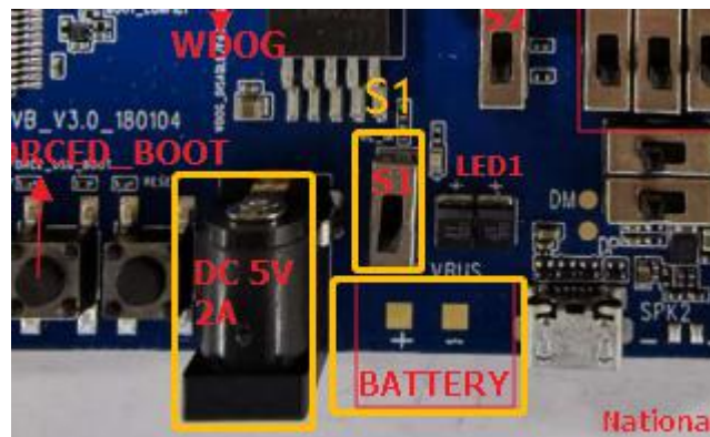
Figure 3-1: L720 development board power in Status (orange Power LED Light up)
