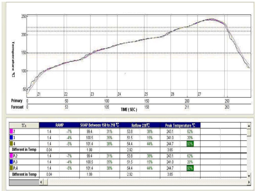
Figure 6-2: Recommend reflow temperature profile
