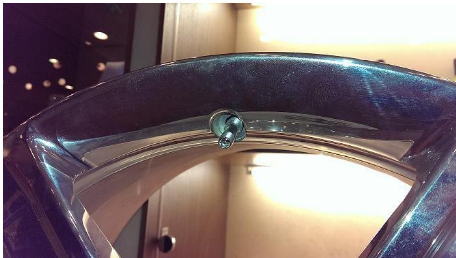
Hold the sensor body against the rim and install then tighten the screw to 20 in-lb
