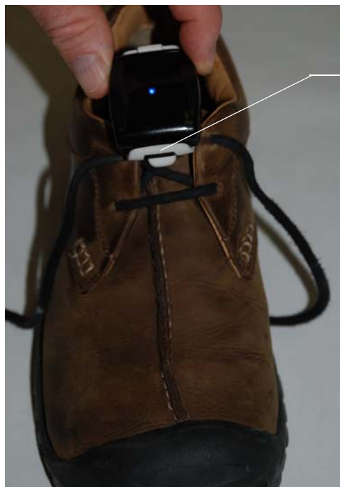
Figure 66. Attaching the IMU/Shoe Clip to the Client's Shoe
