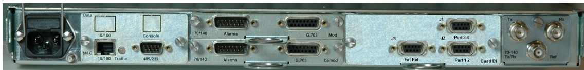
Configuration #3 Modem 1 with G.703 T1/E1 Balanced (DB-15) and Quad E1 Interface Module, 1-4 Ports of E1, with D&I (2) DB-9F)
