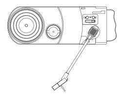
3 Move the TONE ARM from the ARM REST and position it over the 45rpm adapter and align the TONE ARM with the grooves in the 45rpm adapter as shown below.
