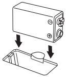
3 Tuck the battery back into the battery compartment and replace the battery cover.
