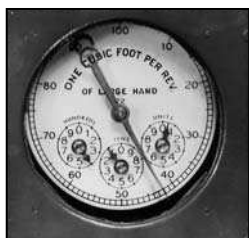
Figure 10 Dials of Typical Gas Meter
