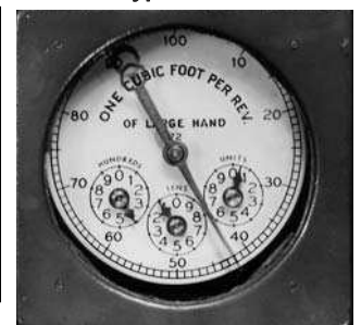
Figure 10 Dials of Typical Gas Meter
