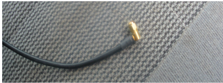
Figure 2.23 Terminated End of Cable 302202
