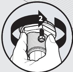
Install mounting screws (K) into mounting nut (J).
