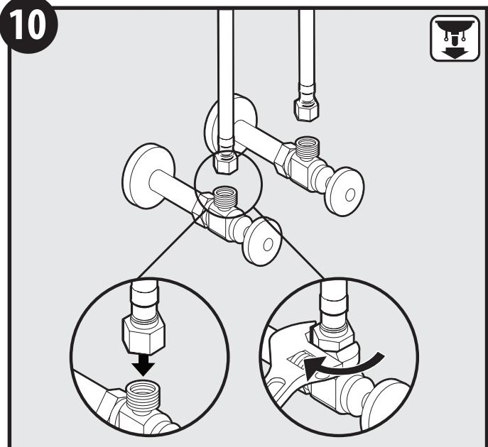
Attach flexible lines to shut off valves. Tighten with wrench.
