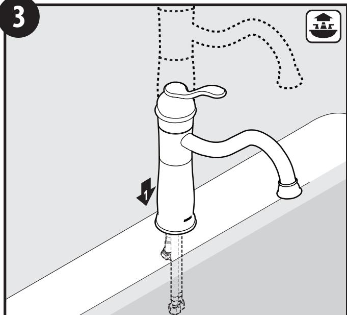
For Single Hole Applications: Place faucet onto mounting surface.
