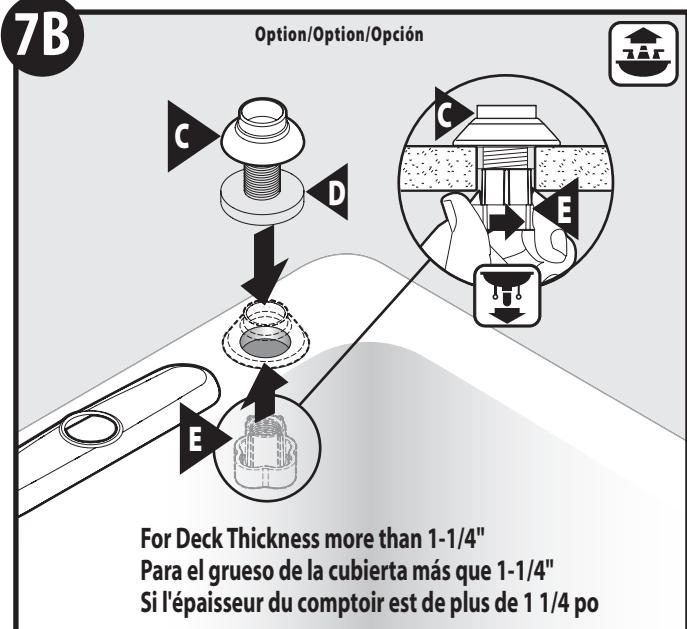
**For Thick Deck Installations:** Place hose guide gasket (D) onto hose guide (C). Place into mounting surface hole. Orient hose guide nut (E) with small end and facing up and tighten to hose guide (C).
