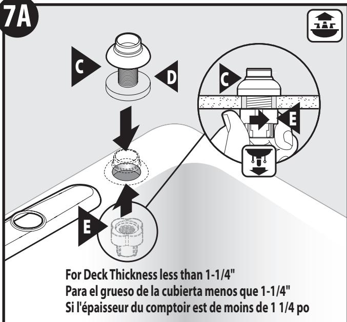
**For Thin Deck Installations:** Place hose guide gasket (D) onto hose guide (C). Place into mounting surface hole. Orient hose guide nut (E) with large and facing up and tighten to hose guide (C).
