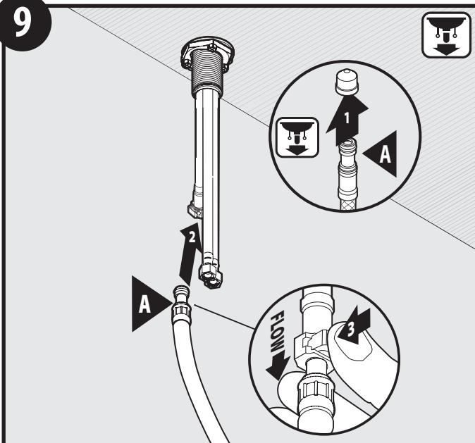
Insert side spray hose (**A**) into hose guide (**C**) until side spray assembly is seated in the hose guide.
