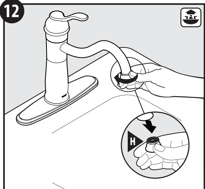
To flush debris from the plumbing system: Remove aerator (H) by unthreading by hand.
