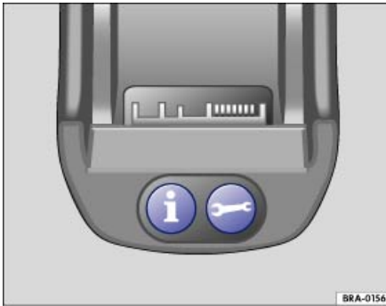
Fig. 8 Charging base with buttons for information call and breakdown call.
