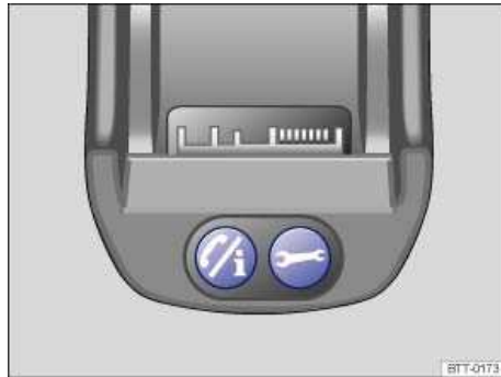
Fig. 6 Charging base with buttons for information call and breakdown call
