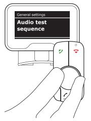
Turn **(**) to select Audio test sequence, and press **(**) to perform the test.
