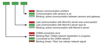
Note 1: The CGW2 resets itself after receiving new configuration from the server (ex. new HB), LED1 starts with RED and the reset cycle continues till all 3 LEDS are GREEN
