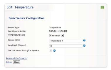
The sensor configuration window allows you to set the primary configurations for each sensor. Within this window you can change the name of the sensor, set the heartbeat (how often the sensor checks-in with the software - default is every 10 minutes), and change the unit of measurement. When you have finished making changes, press the "Save" button at the bottom of this section.
