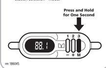
2. Press buttons 1 or 2 (also identified as '+' and '-') to scroll FM radio frequencies up or down.
