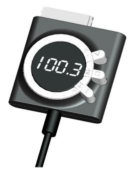
Note the three push buttons. Button-1 is also the "M" button. Button-2 is also the "D" button. Button-3 is also the "S" button.
