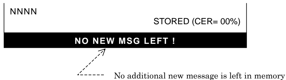
Figure 2-8 Indication of All New Messages Being Acknowledged
