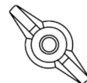
Figure 7-6 Cabinet Ground Terminal
