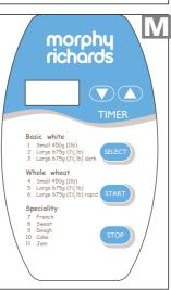
7 Press START. The baking time in hours and minutes will appear in the display. For example, if you chose a recipe using setting 1,
