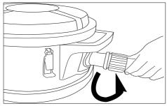
clockwise until it clicks.Make sure it is securely in place. The appropriate cleaning tool can be attached directly to the other end of the suction hose.
