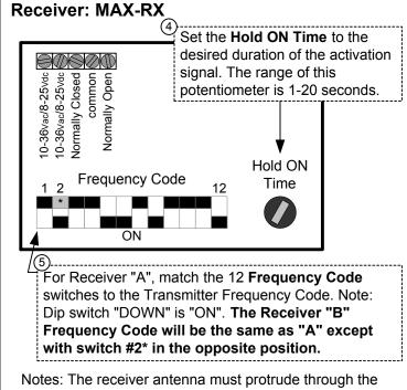
Notes: The receiver antenna must protrude through the operator housing. The maximum relay capacity is 1A @ 120Vac / 30Vdc.
