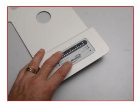
8. Plug the RJ45 Battery Gauge cable into the jack, through the hole in the back of the Battery Gauge housing.
