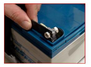
17. Make sure battery connections are tight on both batteries
