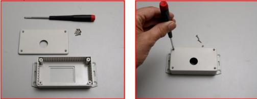
7. Assemble the Mounting plate and Battery Gauge
