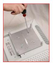
4.4 Attach the Flush Tilting VESA Mount bracket to the back CPU VESA Mount plate
