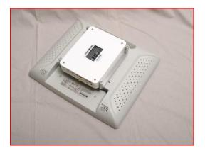
4.6 Attach the back CPU VESA Mount plate to the front CPU VESA Mount plate, using the threaded metal spacers attached to the front plate
