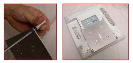
4.2 Place nylon spacers over the Monitor VESA Mount plate threaded inserts where arrows indicate
