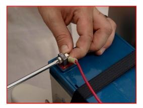
16. The unpainted side of the thermal sensor must be in contact with the battery post.
