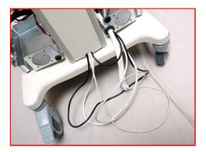
14. Dress the cables at the bottom of the column using corrugated cable wrap, securing with cable ties, and pulling the excess cable length into the sheet metal base.
