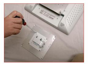
4.5 Place the Media Wave Computer onto the front CPU VESA Mount plate, evenly spaced between the metal spacers and connectors facing down
