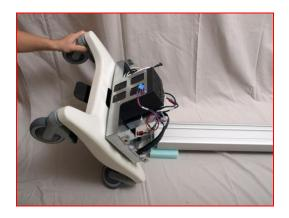
2.3 Insert bolts through the bottom of the cart into the column. Thread each bolt before fully tightening any bolt. Tighten all four bolts.
