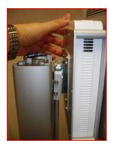
5.1 Position the VESA Mount bracket about one inch from the top of the column rail and secure by tightening the set screws
