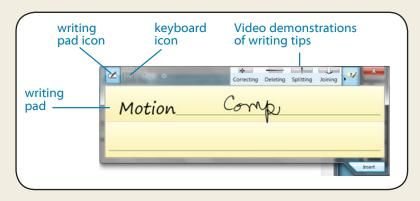
Use the handwriting recognition application to train the C5m/F5m to recognize your handwriting style. To start the application, open Motion Dashboard, tap **Pen & Tablet**, tap **Pen & Input Devices**, and then tap the **Handwriting** tab.
