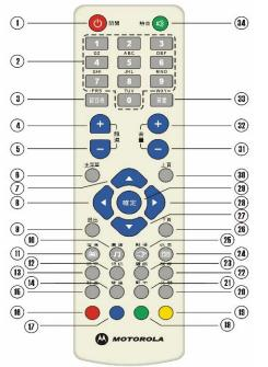
The **MDV850T's remote control** is specially designed to enable you to enjoy your service. All functions of the **MDV850T** can be achieved with this remote control; some functions can be realized on the front panel of the unit as well.
