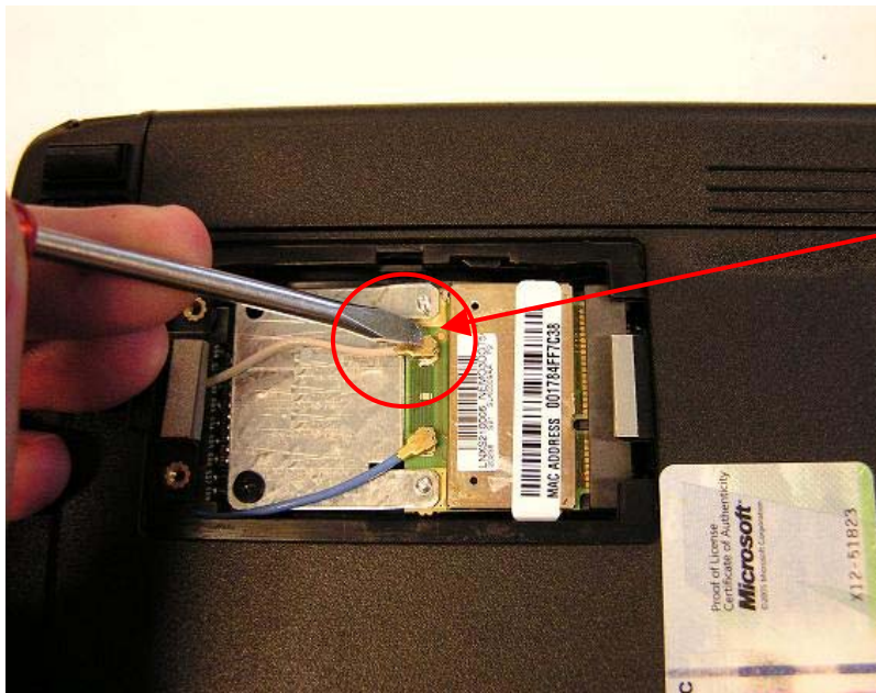
Figure 3-15 Connecting Internal Antennas to the WTM1100 Card.
