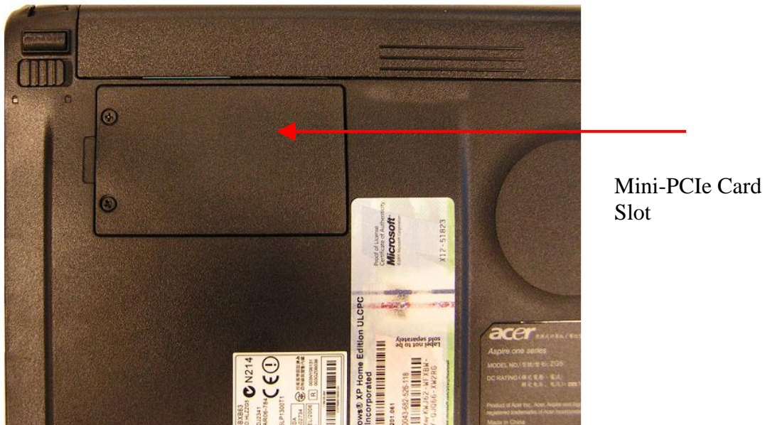
Figure 3-12 Locating the Mini-PCIE Card Slot
