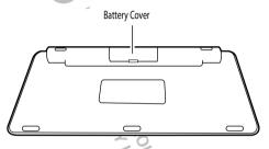
2 Insert 2 "AA" batteries like shown inside compartment and replace cover.
