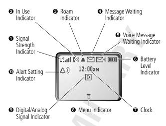
• Signal Strength Indicator Shows the strength of your phone's connection with the network.
