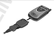
3 Plug the other end of the cable into the serial interface connection on the external device and tighten the screws.
