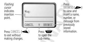
When you enter text, the flashing cursor changes to a *block cursor*, and the soft key functions change:
