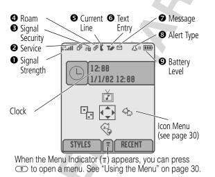
**O** Signal Strength Indicator Shows the strength of your device's connection with the network.
