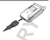
3 Plug the other end of the cable into the serial interface connection on the external device and tighten the screws.
