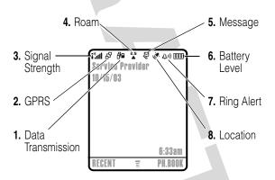
**1. Data Transmission Indicator** Shows connection and data transmission status. Indicators can include:
