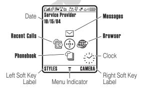
The menu indicator shows that you can press to open the menu. Soft key labels show the current soft key functions. For soft key locations, see page 1.
