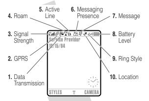
1 Data Indicator – Shows connection status. The Bluetooth® wireless connection indicator ≱ shows when a Bluetooth connection is active. Other indicators can include:
