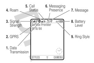
1. Data Transmission Indicator – Show connection and data transmission status. The Bluetooth<sup>®</sup> wireless connection indicator shows when a Bluetooth connection is active. Other indicators can include:
