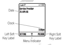
The *Menu Indicator* shows that you can press **I** to open the menu. *Soft Key Labels* show the current soft key functions. For soft key locations, see page 1.
