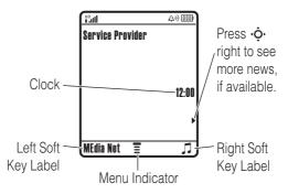
The *Menu Indicator*  $\overline{\equiv}$  shows that you can press  $\Box$  to open the menu. *Soft Key Labels* show the current soft key functions. For soft key locations, see page 1.
