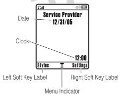
The *Menu Indicator* **T** shows that you can press **T** to open the menu. Soft Key Labels show the current soft key functions. For soft key locations, see page 1.
