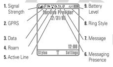
1 Signal Strength Indicator – Vertical bars show the strength of the network connection. You can't make or receive calls when in the strength shows.
