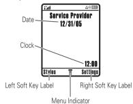
The Menu Indicator shows that you can press to open the menu. Soft Key Labels show the current soft key functions. For soft key locations, see page 1.
